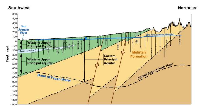
Figure ES-6 Cross Section of Hydrogeologic Framework
